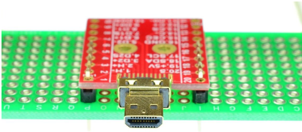
Figure 4: Solid Mounting on prototype PCB
